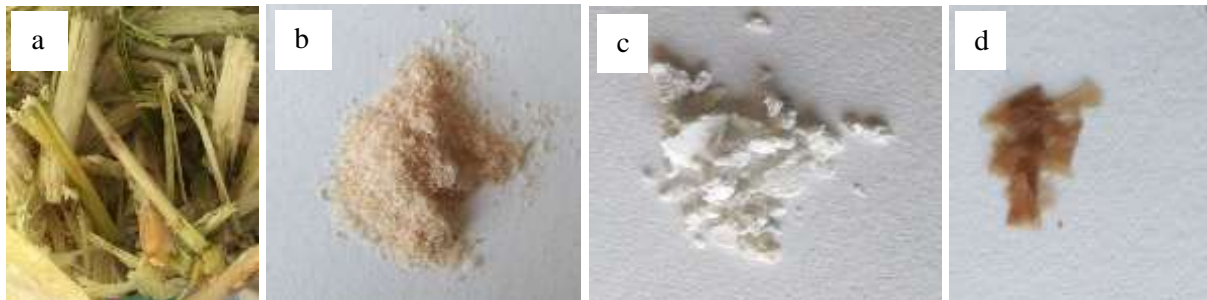
Fig 1. a) Sugarcane bagasse (SB); b) SB after alkali treatment; c) Cellulose (C-SB); d) Nanocellulose (NC-SB)
